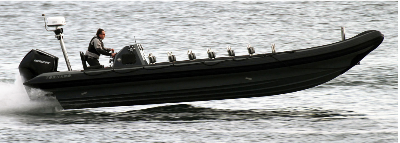
Tornado 9.5m High Performance fitted with twin Mercury Verado 300HP running at high speed
