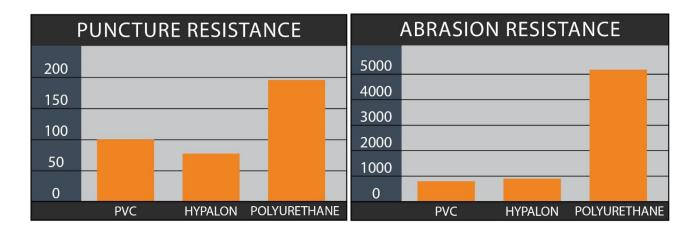
In 1993 the U.S. Navel Surface Warfare Center did a study on polyurethane and the advantages of using it for Rigid Inflatable boats.
